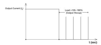
Additionally, if the Io is <105-180% but >100% for a prolong period of time (depending on the load), the Over Temperature Protection (OTP) will be activated due to high temperature on critical components. The power supply will then go into "Latch-off mode" until the PSU cools down and the AC power is recycled.
