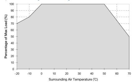
Fig. 1 De-rating for Vertical and Horizontal Mounting Orientation -20°C to -10°C de-rate power by 1% / °C, -10°C to 0°C de-rate power by 2% / °C,
