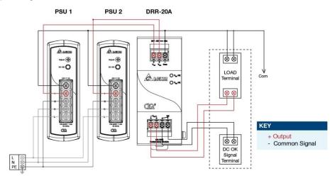
Fig. 2 Redundancy / Parallel Operation Connection Diagram
